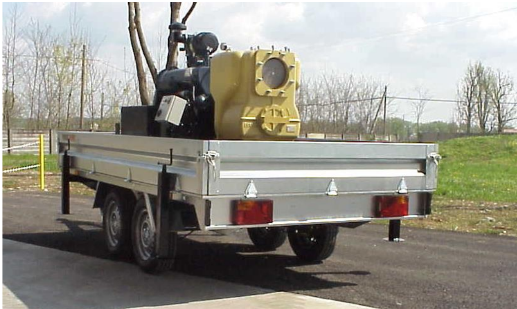
Gruppo motopompa montato su carrello stradale Motor pump unit mounted on a road trolley Groupe motopompe monté sur chariot routier
